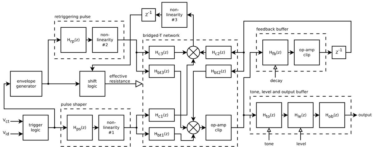
Figure 2: TR-808 bass drum emulation block diagram.
