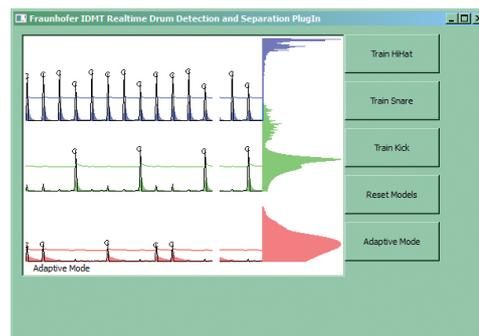
Figure 6: Screen-shot of a VST plug-in encapsulating the proposed algorithm. The semi-transparent colored curves visualize the extracted  $G$  of the individual drums, the colored spectra on the right show the extracted  $B$ . Blue corresponds to hi-hat, green to snare and red to kick. The individual onset detection functions  $D$  are overlaid as black lines and the dynamic thresholds  $T$  as solid colored lines.
