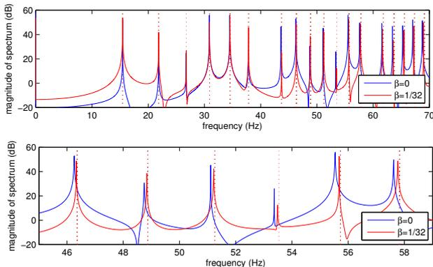
Figure 4: Comparison of low frequency responses for cubic room using IISO1 explicit scheme ( $\alpha_1 = 1/3, \beta = 0$ ) with grid size  $21 \times 21 \times 21$ , and fourth-order implicit scheme ( $\alpha_1 = 1/3, \beta = 1/32$ ) with grid size  $12 \times 12 \times 12$  and  $M = 5$ . Dotted lines denote theoretical modal frequencies.
