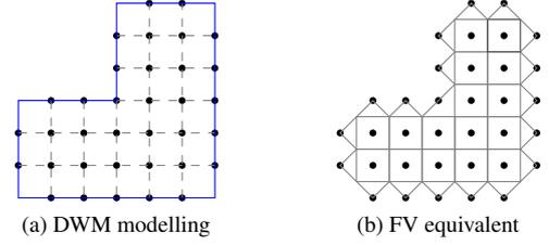
Figure 5: Desired L-shaped domain in blue, modelled using 1-D DWM boundaries (left) and equivalent FV interpretation (right). Dashed lines indicate connectivity, or DWM delay lines. Notice that adjacent boundary nodes are not interconnected, in both cases.
