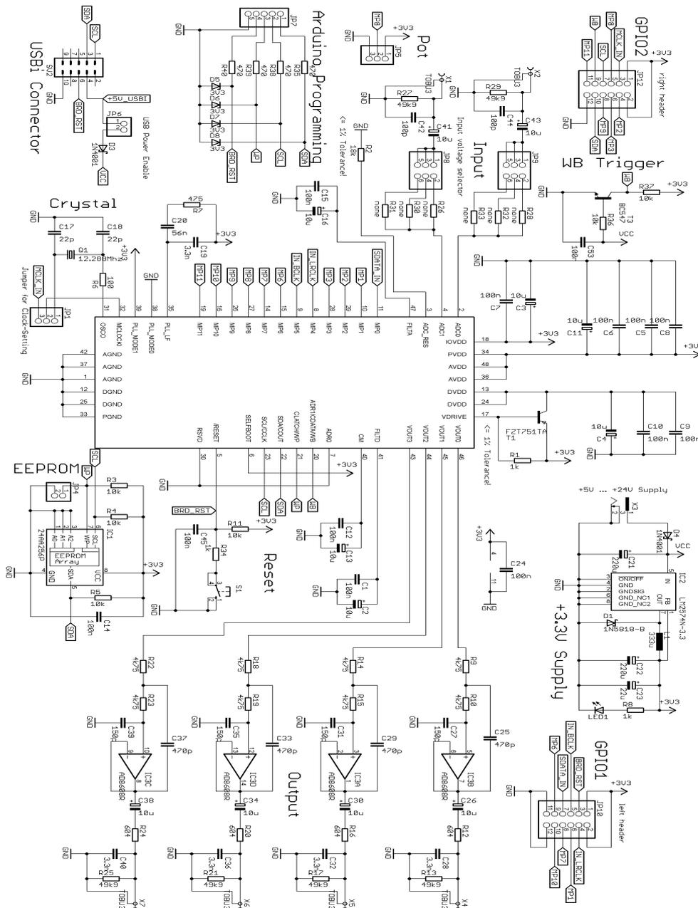
Figure 2: Schematic of the freeDSP board version 0.3.
