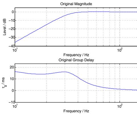
Figure 5: Original Magnitude and group delay response of the loudspeaker
