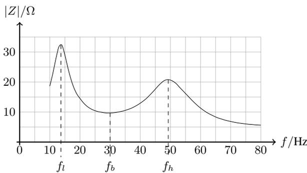
Figure 2: Impedance curve of a vented box
