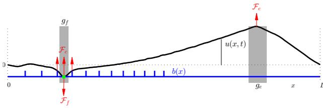
Figure 1: Diagram of string, of displacement  $u(x, t)$ , in contact with a barrier  $b(x)$ , as indicated in blue. An excitation force density  $\mathcal{F}_e$  is applied over a distribution  $g_e$ , and a force density  $\mathcal{F}_f$  is applied by a finger (indicated in green) over a distribution  $g_f$ . A collision force density  $\mathcal{F}_c$  results at points of contact between the string and barrier.
