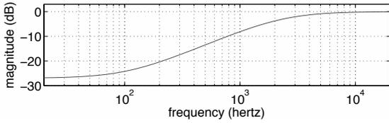
Figure 4: Pulse shaper shelf filter core, magnitude response.
