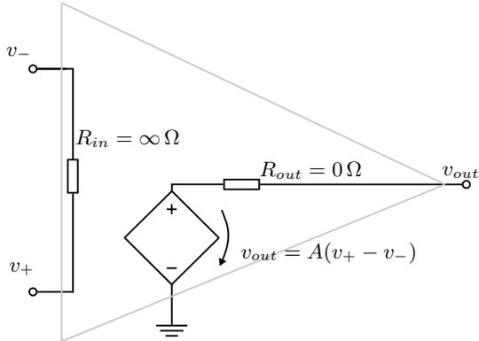
Figure 2: Equivalent circuit diagram for an operational amplifier.
