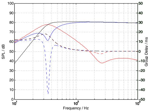
Figure 1: Spice simulation of vented box showing magnitude (—) and group delay (---) responses of the driver (blue), the port (red) and the combined output (black).
