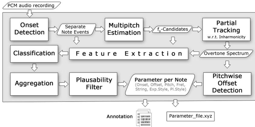
Figure 2: Schematic model of the analysis framework.
