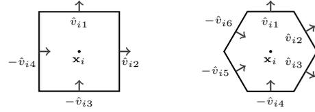
Figure 3: Square and hexagonal cells for staggered grid (FDTD) schemes
