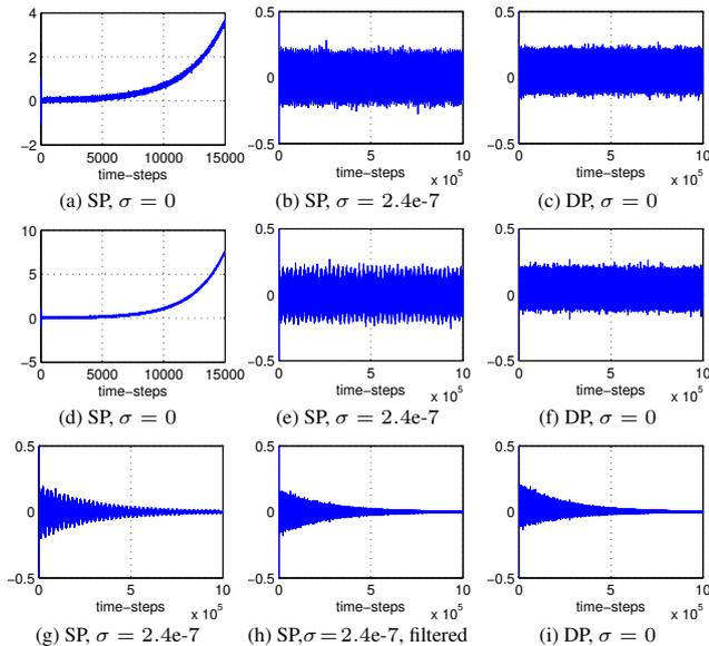
Figure 6: Responses from cubic box obtained using explicit/implicit schemes with  $\alpha_1 = 1/3$  in single precision (SP) and double precision (DP), with  $\lambda = 0.9999\lambda_{\max}$  in each case. Implicit schemes use  $M = 8$  iterations. Note that  $\sigma$  is not used in double precision. A DC blocking filter was applied to the output in Fig. 6h.
