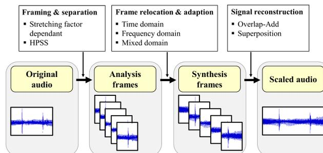
Figure 1: General processing pipeline of TSM procedures.
