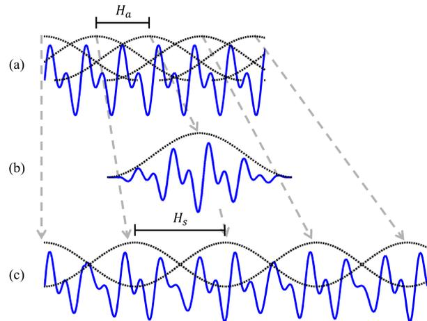
Figure 2: The principle of OLA TSM. (a): Input signal  $x$  (solid line). The analysis frames are indicated by the window functions (dotted lines). (b): One synthesis frame. (c): Output signal as sum of all synthesis frames.
