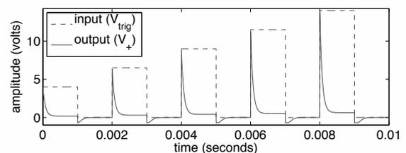
Figure 3: Pulse shaper behavior under various input pulses.
