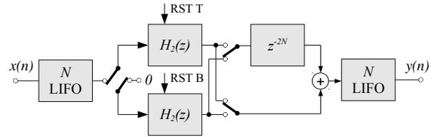
Figure 4: Block diagram of time-reversed filter implementation from [24]
