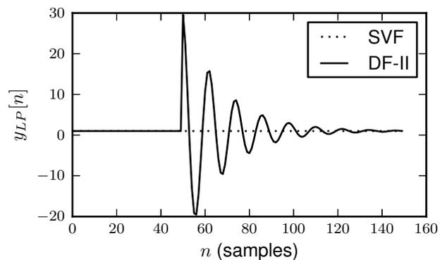
Figure 1: Comparison between lowpass state variable filter and Direct-Form II topology of steady state DC response when parameters are changed. At sample 50, the parameters are changed from  $g = 0.0458$  and  $R = 0.4545$  to  $g = 0.2679$  and  $R = 0.1111$ .
