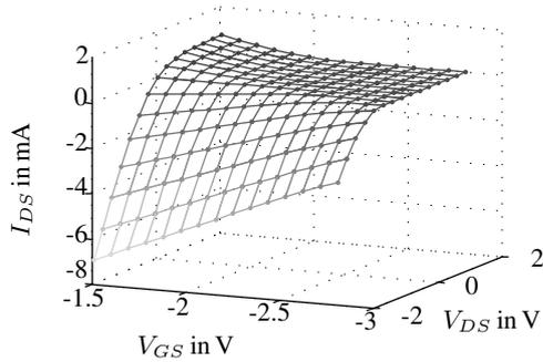
Figure 5: Output characteristic of a single JFET.
