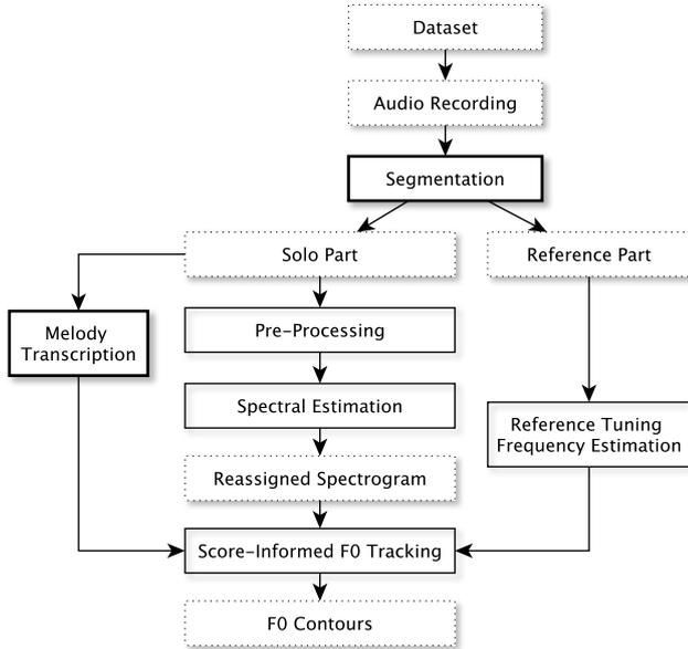
Figure 1: Flow-chart of the proposed algorithm for score-informed  $f_0$ -tracking. Steps illustrated with thicker outline are performed manually, all other processing steps are performed automatically.
