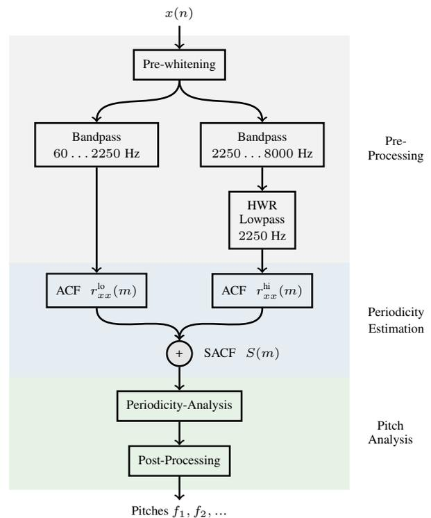
Figure 1: Block diagram of the presented pitch detection algorithm.
