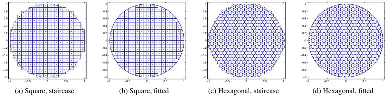
Figure 6: Finite volume tilings representing circular plate of radius one. Square and hexagonal staircase and fitted tilings.
