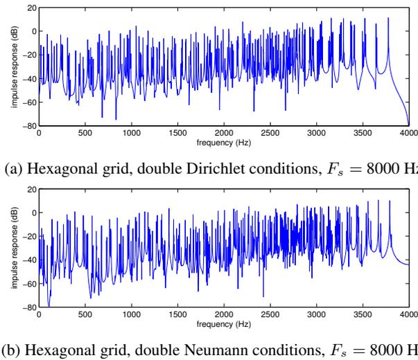
Figure 9: Impulse response spectra from circular plate
