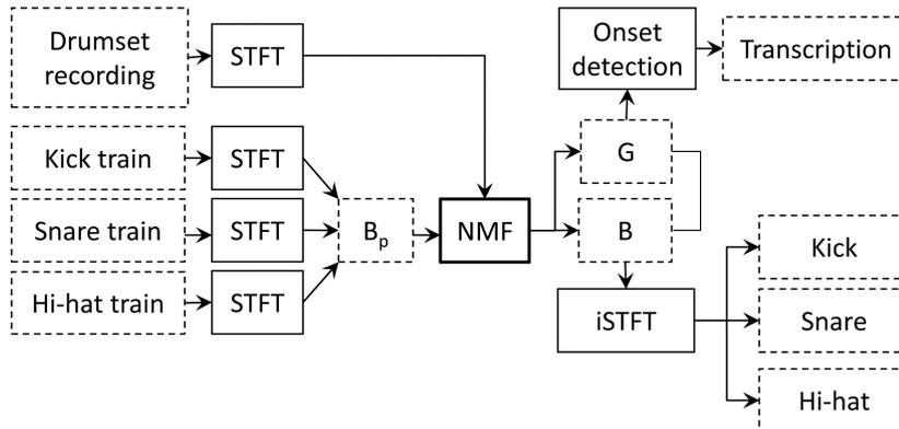
Figure 3: Overview of the proposed method. Prior basis vectors  $B_p$  are derived from isolated drum sound spectrograms. Drum set recordings are split into spectral frames individually subjected to NMF. The resulting  $B$  and  $G$  are used for onset detection as well as inverse STFT in order to obtain isolated drum instrument recordings.
